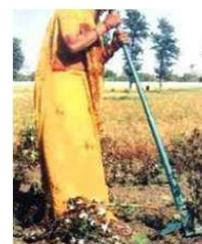
original position with help of a tension spring fitted between press plate and mainframe. The unit can easily be moved to next plant with the help of ground wheel. Field capacity of this equipment is about  $280 \text{ m}^2/\text{ha}/\text{hr} = 0.027 \text{ hr}$ . Its cost is about Rs. 1800/-.
